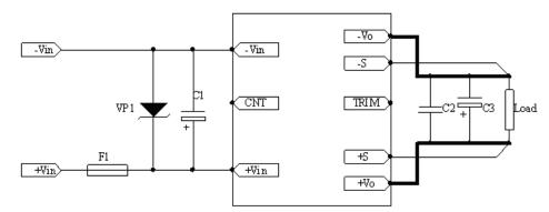
Notes: The basic connection indicates the basic requirements that the power module can provide rated output voltage and rated power only, Please refer the instruction followed for further information.
