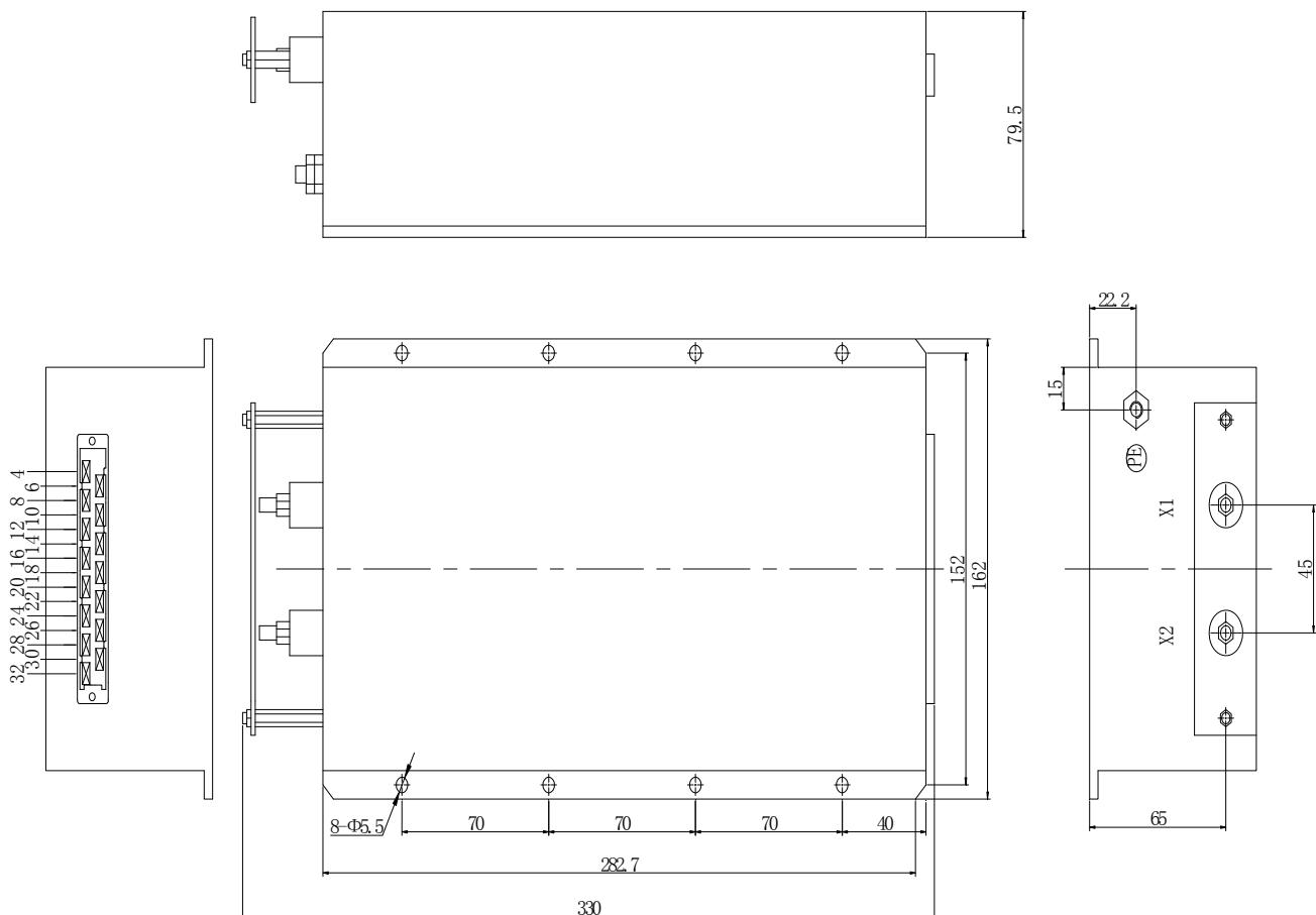
Input 900-2000Vdc Output 110V/3.7A
